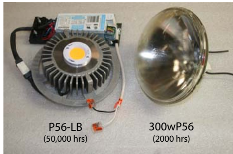
P56-LB LED Par Lamp Retrofit next to the incandescent 300w Par lamp it is replacing.
